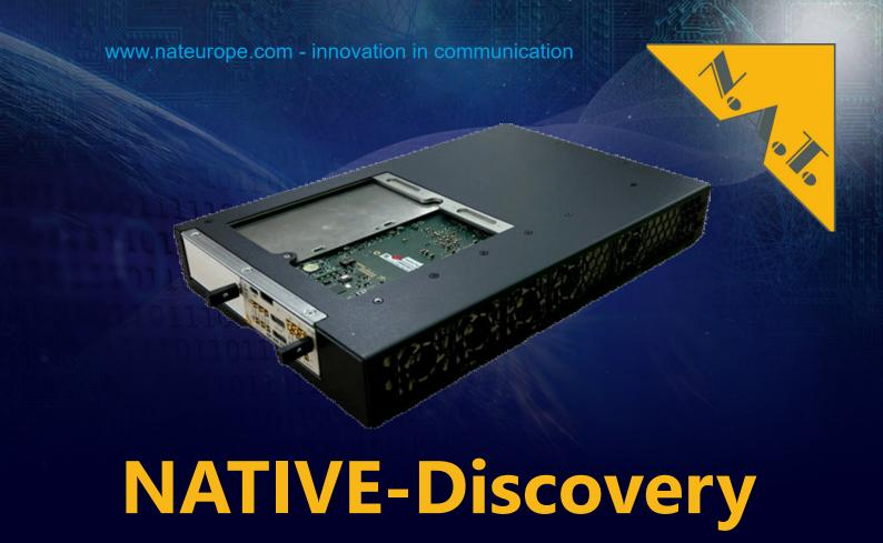
The **NATIVE-Discovery** is a one slot MTCA.0 chassis AMC box with minimum MTCA infrastructure including cooling as well as basic management and switching functionality. The system is powered by an external power supply.
