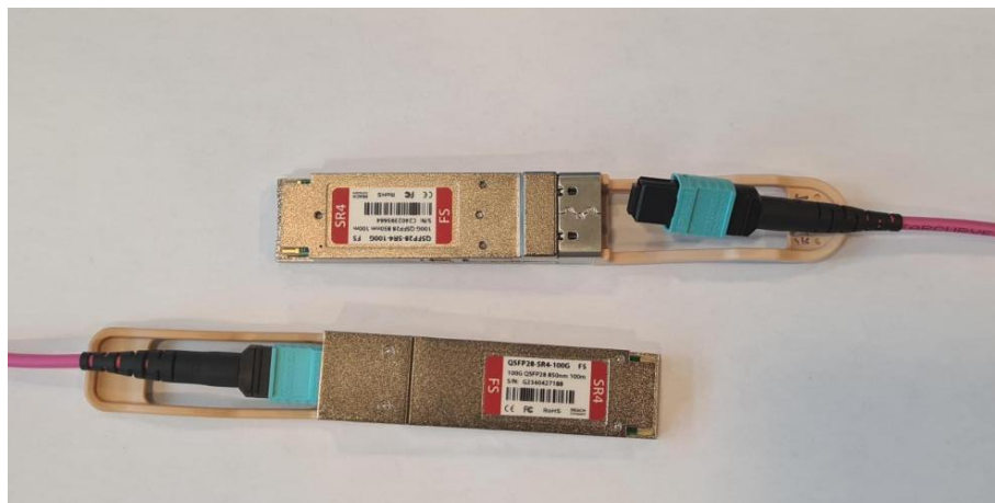
Figure 6 – QSFP28: MPO – MPO Cable for SR4 Transmission Mode
