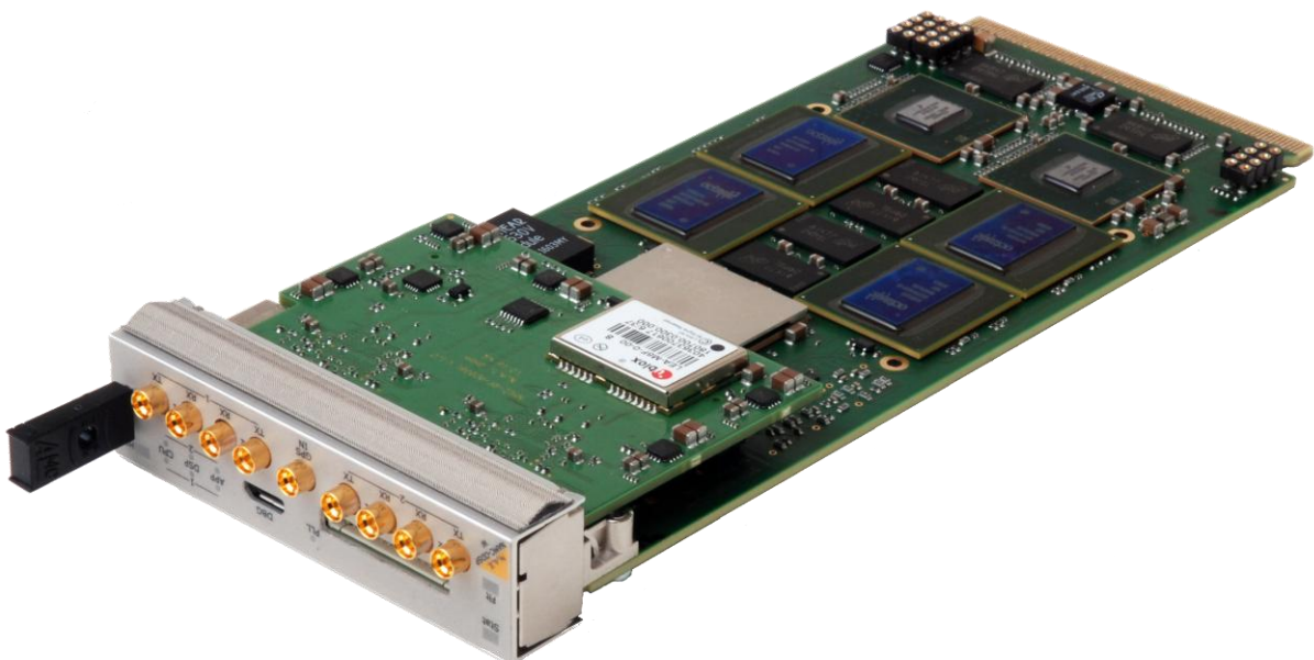
Figure 1: NAMC-ODSP-W with attached NMEZ-RF-AD9361
