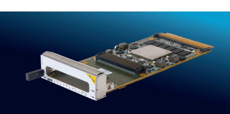
The NAMC-ZYNQ-FMC is an AdvancedMC (AMC) featuring a Xilinx ZYNQ®-7000 FPGA and an FPGA mezzanine card (FMC) slot. This single-width, mid-size AMC is designed for data acquisition and processing applications and computing nodes. The ZYNQ-7000 FPGA provides the software programmability of an ARM®-based processor with the hardware programmability of an FPGA, enabling key analytics and hardware acceleration while integrating CPU, DSP, ASSP, and mixed signal functionality on a single device.
